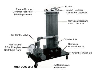
Sethco centrifugal filter systems are shipped fully assembled, completely tested and ready for start-up and continuous operation. Each system includes a CPVC filter chamber, a PP or fiberglass pump, corrosion resistant panel, flow control valve and filter media. All systems are suitable for temperatures to 180° F. All motors are continuous duty, totally enclosed, fan cooled.
